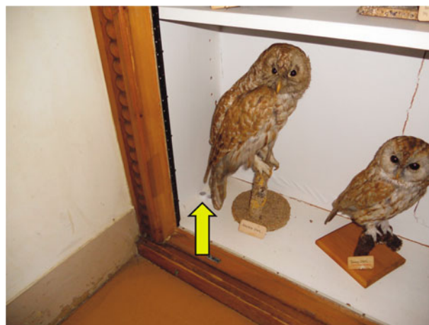
Figure 3: Badge samplers (arrow) measuring organic acids placed, down to the left, in one of the Osborne Swiss Cottage showcases.
